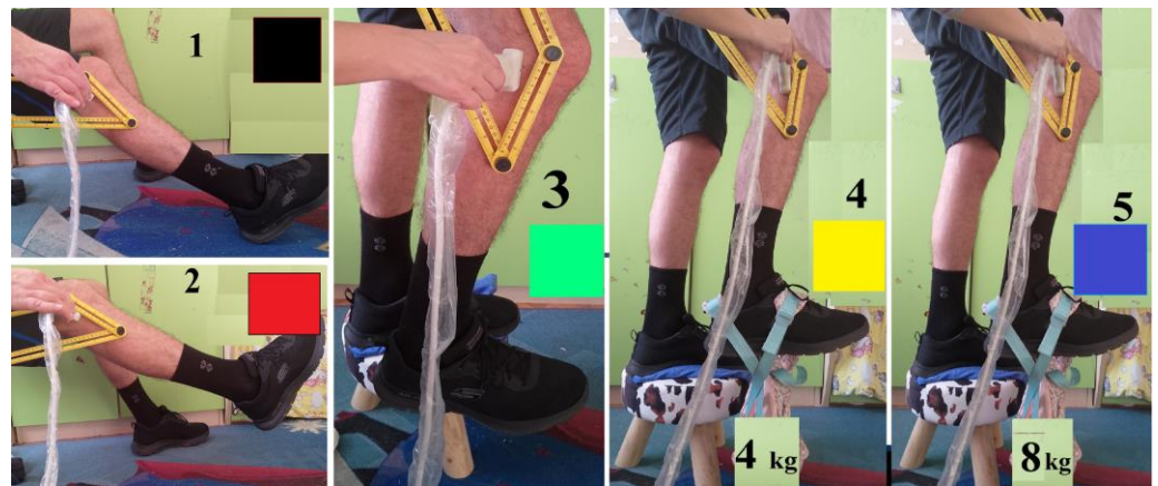
Figure 2. Stage 1 experimental setup showing lower limb poses with loads. The colors show the 5 different lower limb poses used to achieve different knee joint responses.
