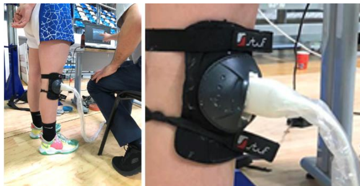
Figure 4. Experimental setup in stage 3, with ultrasound transducer muff to immobilize the transducer on the knee joint.
