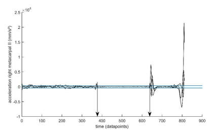
**Figure 2.** Time normalization of the aiming phase. When all components of the acceleration of the right-hand metacarpal II (black traces) remained between -400 and  $400 \text{ mm/s}^2$  (blue lines) for at least five consecutive time samples, the start of the aiming phase was defined (left vertical arrow), and release was defined when this condition was no longer met (right vertical arrow).
