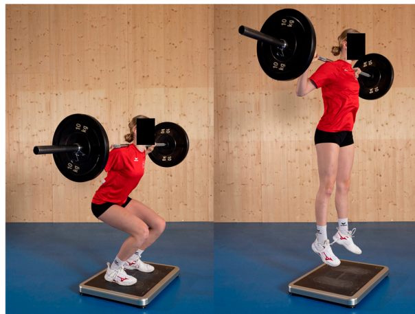
Figure 3. The squat jump test, executed with additional external load, performed on a force plate to assess lower-body power.
