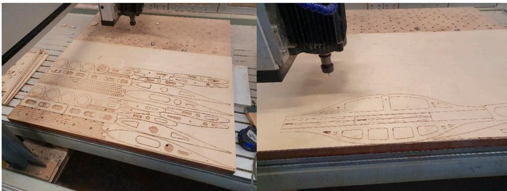
**Figure 15.** Cutting out the elements that will constitute the interior structure.
