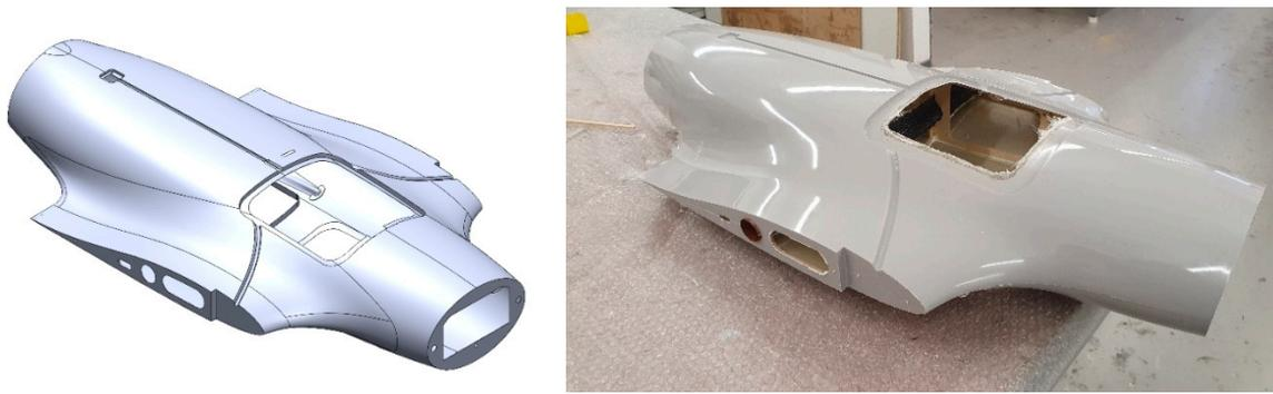
**Figure 17.** Three-dimensional and physical model of the fuselage skin.
