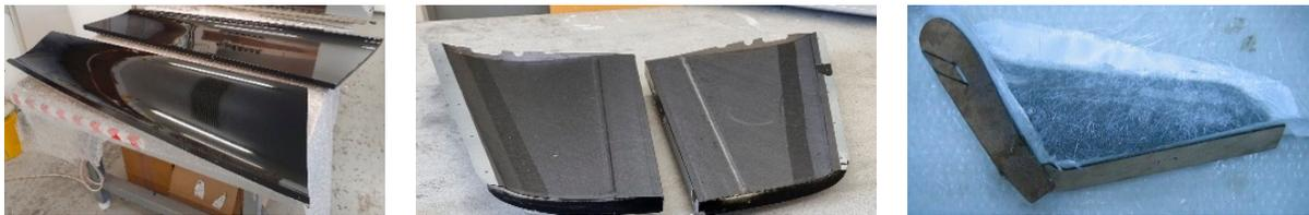
**Figure 18.** Molds for the three sections of the wing.
