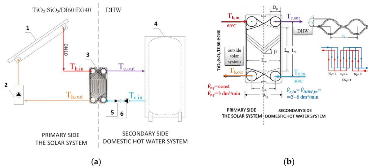
**Figure 2.** (a) The hydraulic scheme of the solar system including the plate heat exchanger and operating conditions; (b) initial conditions of the solar system and basic dimensions of a chevron-type PHE with its cross-section dimensions normal to the direction of troughs.
