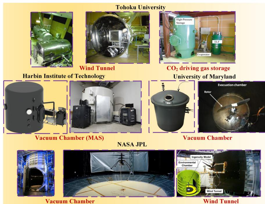
Figure 7. Mars atmospheric environment simulation setups.
