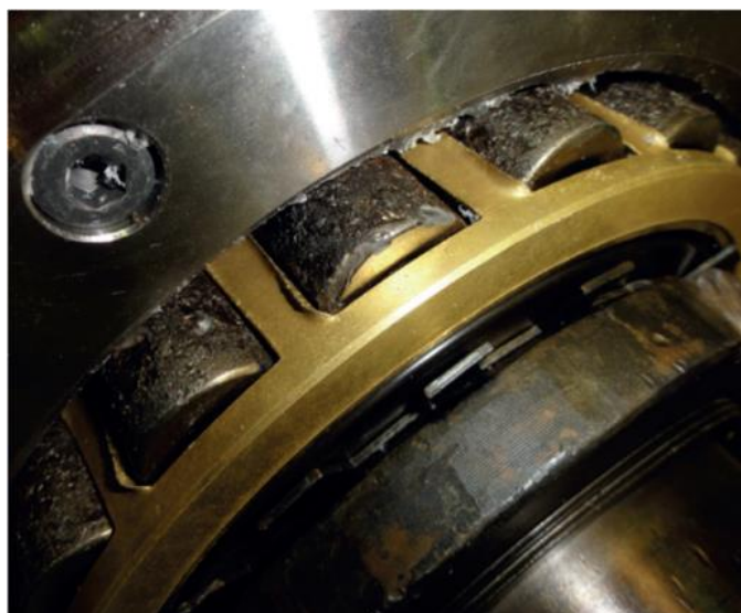
Figure 1. Visualization of failed bearings in EVA autoclave reactor.
