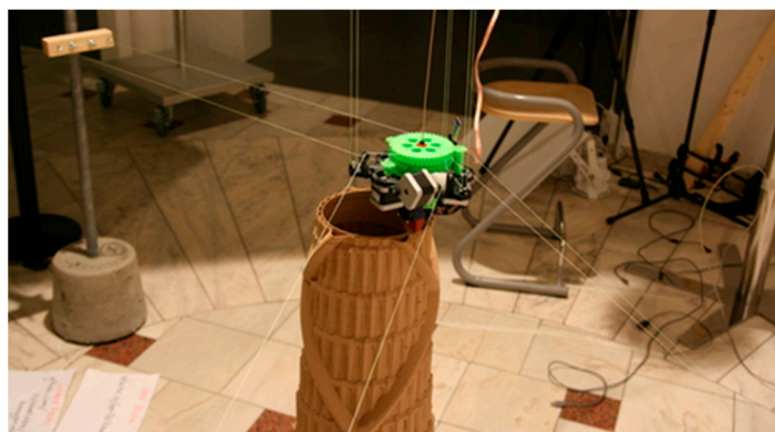
Figure 1. Hangprinter in operation printing a Babel tower. Reprinted under Gnu Free Documentation License by Torbjørns from Ref. [83].
