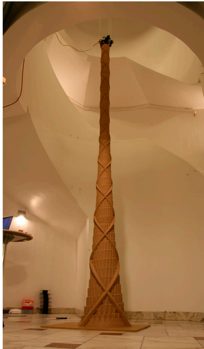
Figure 2. The open-source hangprinter being used to construct a multi-story building model. Reprinted under Gnu Free Documentation License by Torbjørns from Ref. [83].
