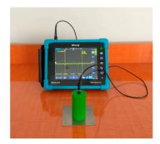
Figure 2. Device for measuring surface energy.
