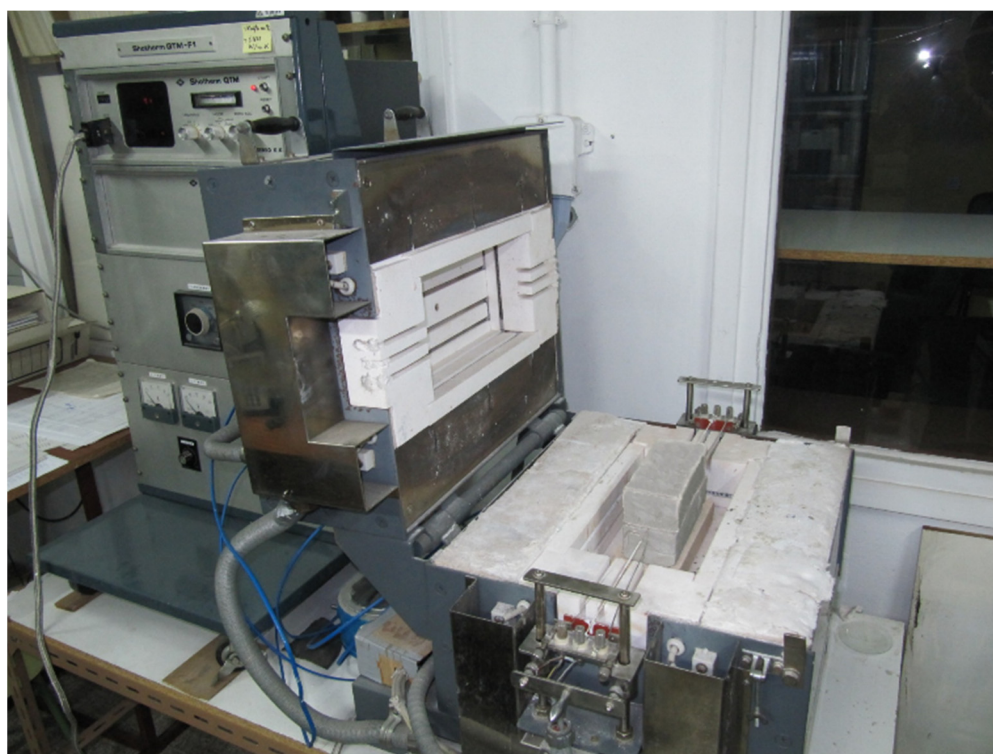
Figure 6. Shotherm QTM-F1 thermal conductivity meter.
