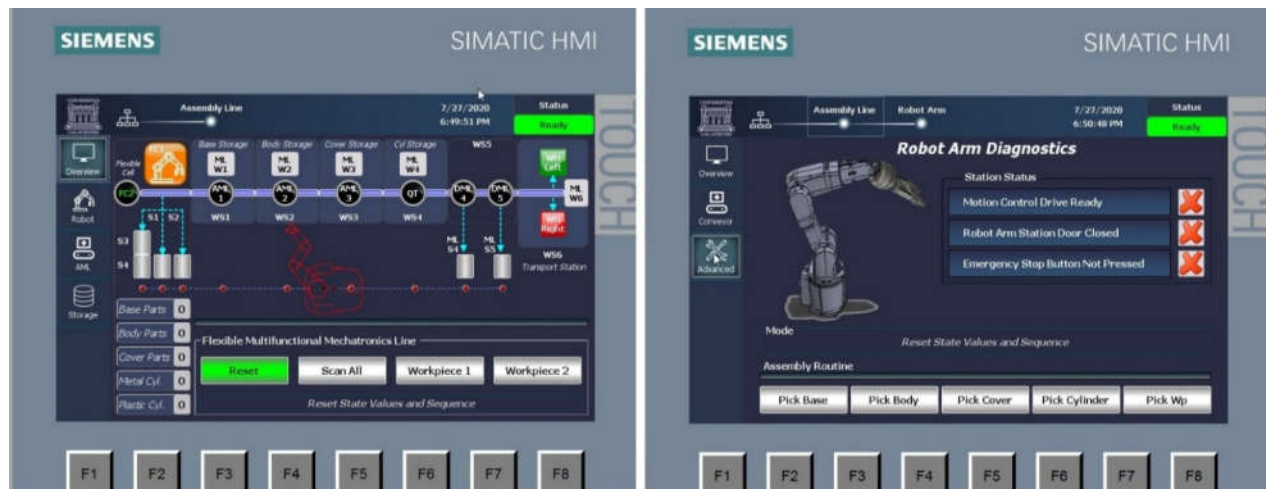
Figure 21. Control and visualization of A/D/RML via Siemens HMI (KTP700).
