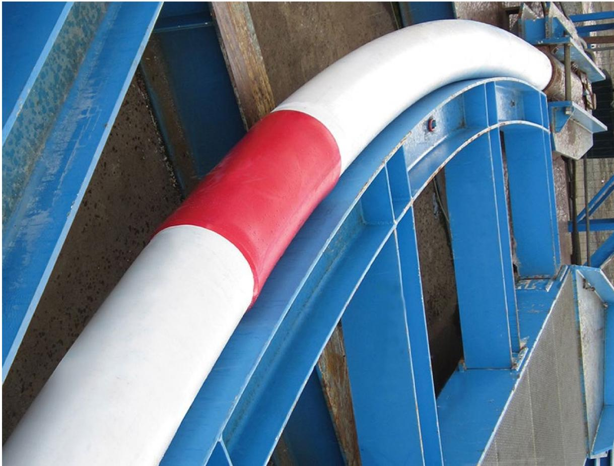
**Figure 2.** Typical example of a reeled system during a bend test for validating reeling capability after coating by Bredero Shaw. (Permission obtained from World Pipelines and Elizabeth Corner. Source: Corner E. [48]).
