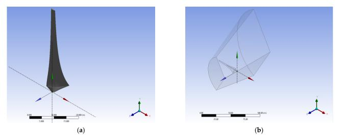
**Figure 2.** (a) Optimum blade constructed with the NREL S809 airfoil; (b) Computational domain over the blade.
