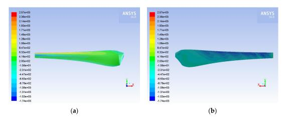
**Figure 12.** Contours of pressure on (**a**) the pressure; (**b**) the suction side of the blade for hailstorm conditions and air velocity equal to  $15 \text{ m} \cdot \text{s}^{-1}$ .
