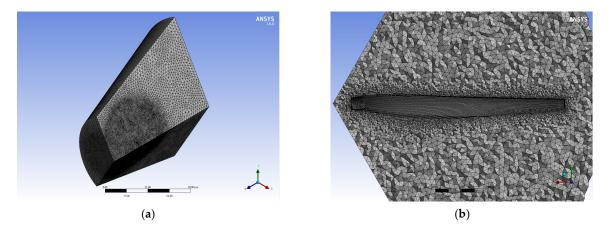
Figure 3. (a) Hybrid mesh and (b) detail of the mesh around the blade.
