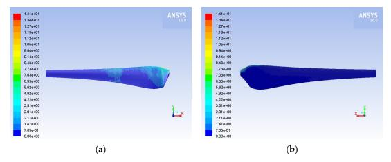
**Figure 13.** Concentration of particles on (**a**) the pressure; (**b**) the suction side of the blade for hailstorm conditions and air velocity equal to  $10 \text{ m} \cdot \text{s}^{-1}$ .
