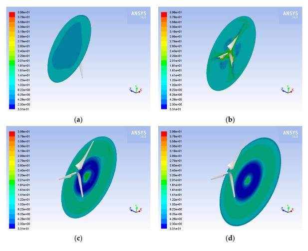
**Figure 5.** Contours of velocity at (**a**) -15 m; (**b**) 0 m; (**c**) 15 m; (**d**) 30 m from the three-bladed HAWT rotor for airflow and air velocity equal to  $10 \text{ m} \cdot \text{s}^{-1}$ .
