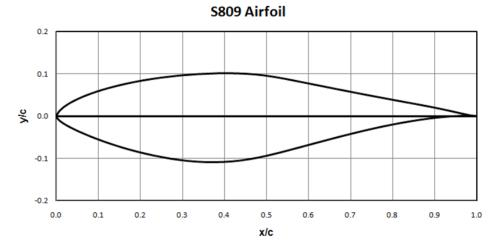
Figure 1. The S809 airfoil and its coordinates in graphical representation [39].
