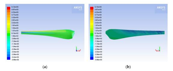
**Figure 8.** Contours of pressure on (**a**) the pressure; (**b**) the suction side of the blade for airflow and air velocity equal to  $15 \text{ m} \cdot \text{s}^{-1}$ .
