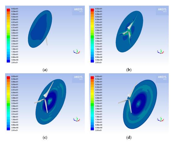
**Figure 9.** Contours of velocity at (**a**) -15 m; (**b**) 0 m; (**c**) 15 m; (**d**) 30 m from the three-bladed HAWT rotor for hailstorm conditions and air velocity equal to 10 m·s<sup>-1</sup>.
