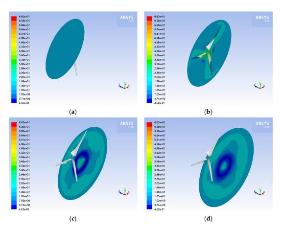
**Figure 10.** Contours of velocity at (**a**) -15 m; (**b**) 0 m; (**c**) 15 m; (**d**) 30 m from the three-bladed HAWT rotor for hailstorm conditions and air velocity equal to  $15 \text{ m} \cdot \text{s}^{-1}$ .
