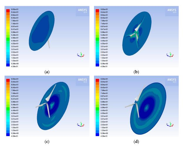
**Figure 6.** Contours of velocity at (**a**) -15 m; (**b**) 0 m; (**c**) 15 m; (**d**) 30 m from the three-bladed HAWT rotor for airflow and air velocity equal to  $15 \text{ m} \cdot \text{s}^{-1}$ .
