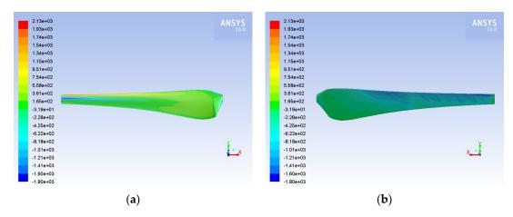
**Figure 11.** Contours of pressure on (**a**) the pressure; (**b**) the suction side of the blade for hailstorm conditions and air velocity equal to  $10 \text{ m} \cdot \text{s}^{-1}$ .
