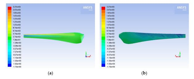
**Figure 7.** Contours of pressure on (**a**) the pressure; (**b**) the suction side of the blade for airflow and air velocity equal to  $10 \text{ m} \cdot \text{s}^{-1}$ .
