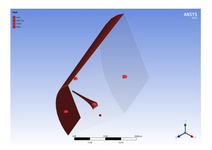
Figure 4. Computational domain and boundary conditions.
