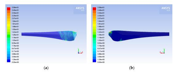
**Figure 14.** Concentration of particles on (**a**) the pressure; (**b**) the suction side of the blade for hailstorm conditions and air velocity equal to  $15 \text{ m} \cdot \text{s}^{-1}$ .
