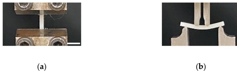
**Figure A1.** Photographs of the P<sub>100%</sub> test pieces in their jigs during loading for the (a) uniaxial tensile test ( $\epsilon_T = 0.05$ ) and (b) four-point flexural test ( $\epsilon_F = 0.2$ ). Bar: 10 mm.
