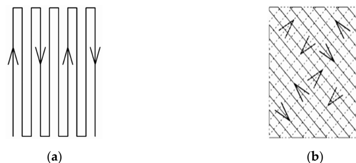
Figure 2. Nozzle scan patterns for the test pieces fabricated with the FFF 3D printer. (a) Parallel, P.; (b) Cross-hatched at opposing diagonal angles, C.
