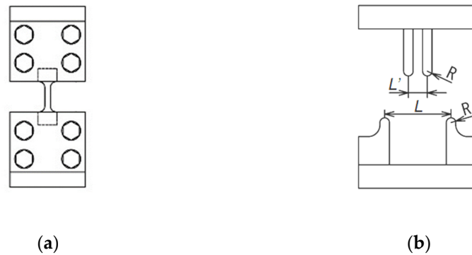
Figure 3. Schematics of the jigs for the (a) uniaxial tensile test and (b) four-point flexural test.
