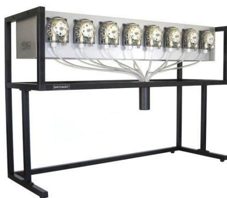
Figure 1. Bartendro bar robot with fifteen peristaltic pumps [6].
