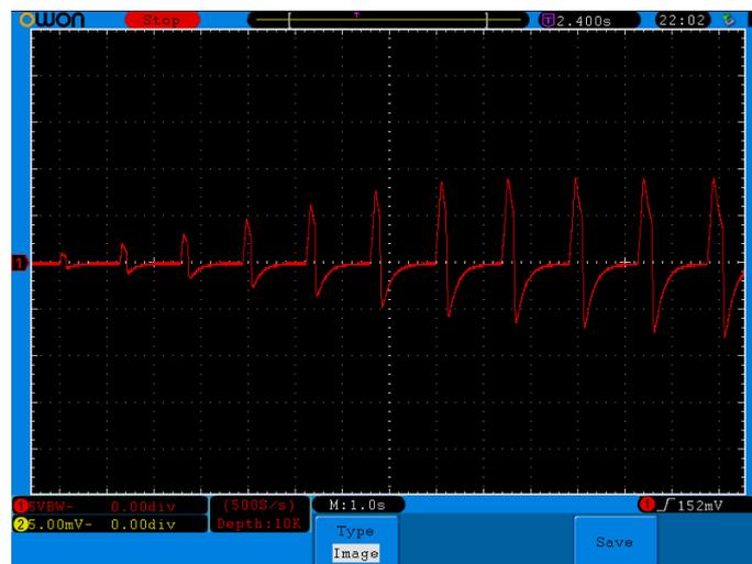
**Figure 5.** Cycling 1 mm per second with increasing travel. Vertical 5 V per cm, Horizontal 1 s per cm.
