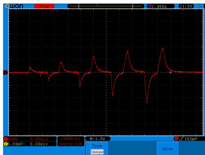
**Figure 6.** Cycling 2 mm per second with increasing force. Vertical 1 V per cm, Horizontal 1 s per cm.
