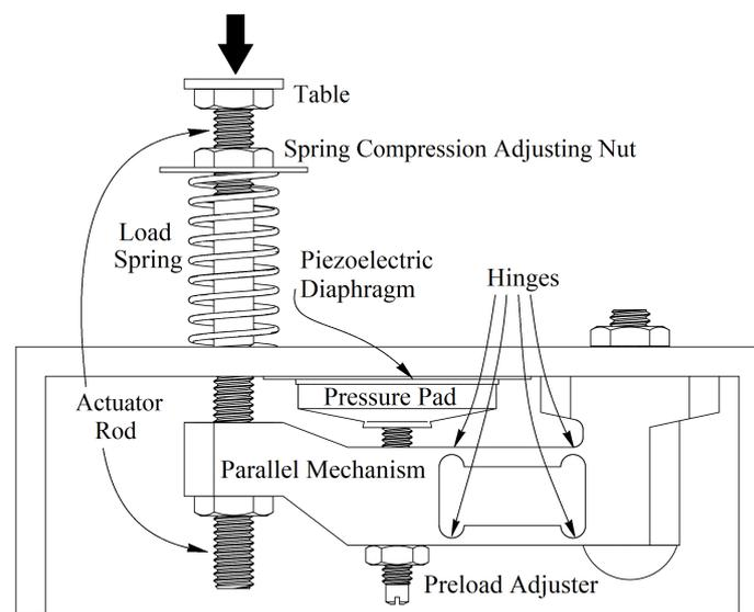
**Figure 2.** Test equipment for obtaining response data.
