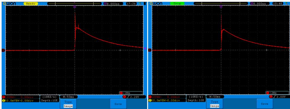
**Figure 7.** Peak amplitude after 1 h (642 cycles) and after 100,000 cycles. Vertical 10 V per cm, Horizontal 50 ms per cm.
