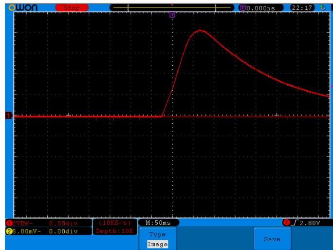
**Figure 4.** Z travel 1 mm per second with pre-travel and after-travel. Vertical 2 V per cm, Horizontal 50 ms per cm.
