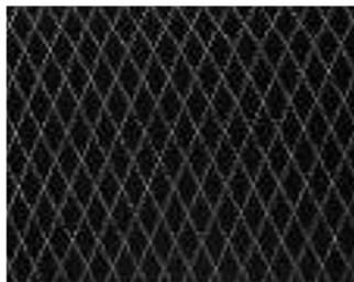
**Figure 2.** Textile electrode used to sense biological signals such as electrocardiography [43].
