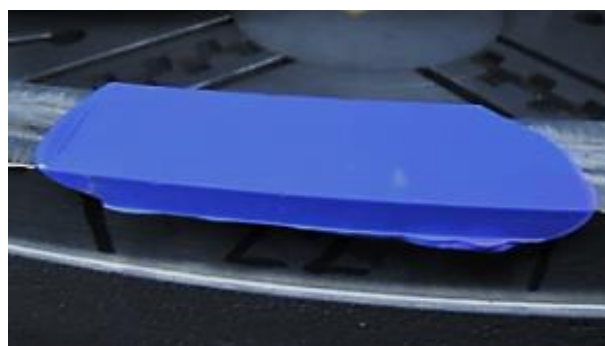
Figure 12. Workpiece surface imprint used for indirect roughness measurements.
