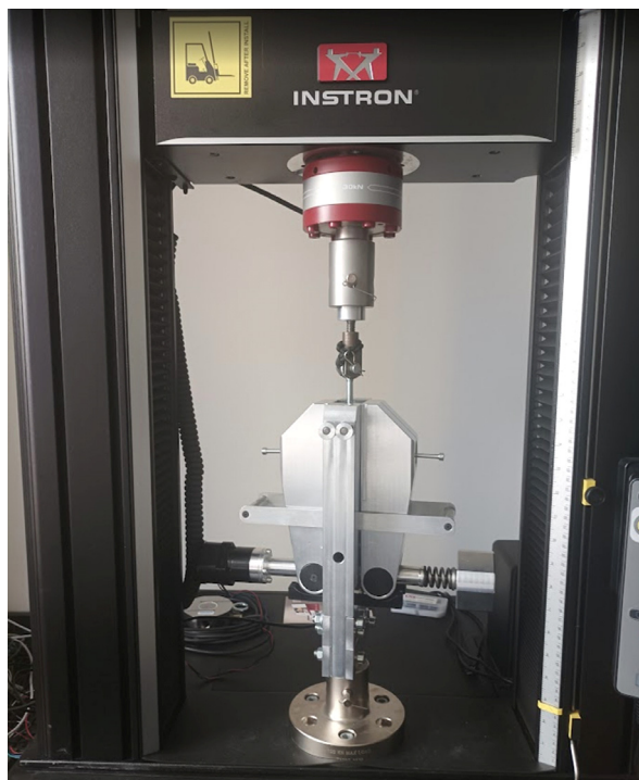
Figure 6. The friction-measuring device mounted on an Instron 68TM-30 universal testing machine.
