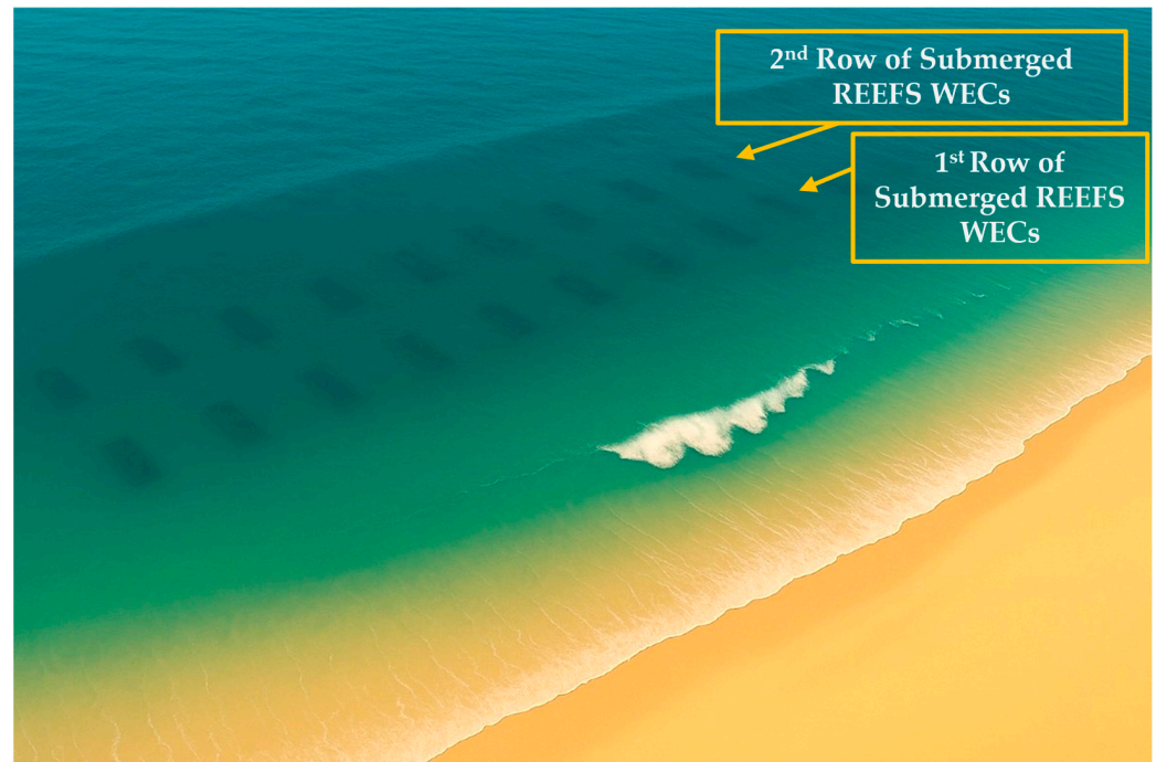
Figure 14. Illustrative projection of a full-scale REEFS WEC nearshore wave farm (concrete version).
