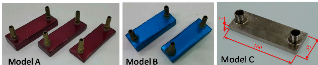
Figure 5. The prototypes of various heat exchangers (unit: mm): the left drawing shows the Model A heat exchangers of three heights; the center shows Model B heat exchangers of two heights; the right is Model C heat exchanger.
