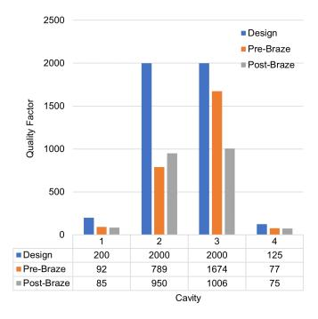
Figure 19. Quality factor of klystron circuit cavities as simulated, before brazing, and after brazing.
