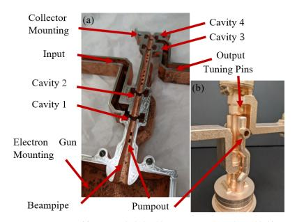
Figure 8. Diagram of features included in klystron circuit. (a) Unbrazed half-piece. (b) Full, brazed circuit.
