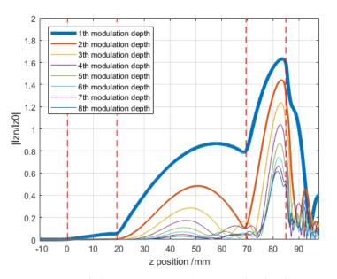
**Figure 2.** First eight harmonic current values normalized to the average beam current as a function of axial distance. Vertical red dashed lines indicate the position of each resonant cavity.
