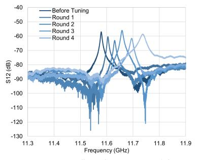
Figure 14. Transmission coefficient of test cavity measured after successive rounds of tuning.
