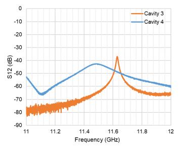
Figure 17. Measured transmission coefficients of cavities 3 and 4 measured after brazing.
