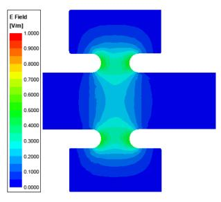
Figure 9. Normalized E-field of Cavity 3 simulated in HFSS.
