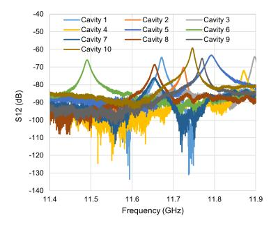
Figure 12. Transmission coefficient of 10 test cavities measured after brazing.
