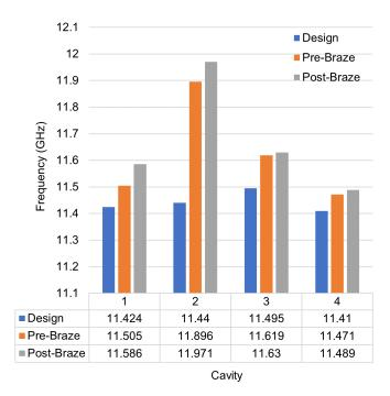
Figure 18. Resonant frequency of klystron circuit cavities as simulated, before brazing, and after brazing.
