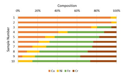
**Figure 6.** Material composition of plated surface measured after brazing with analysis at increasing depths via laser ablation.
