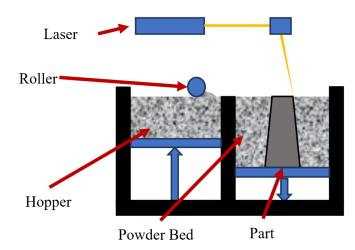
Figure 3. Diagram of DMLS printer.
