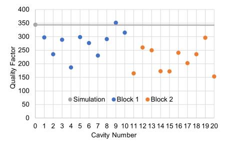
**Figure 11.** Q factor of all test cavities measured after printing. Simulated Q factor is shown as horizontal grey line. Simulated geometry is adjusted to reflect cavity geometry before face machining.
