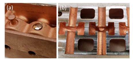
**Figure 16.** Damaged cavity after failed tuning test. (a) Tuning pin head on exterior of cavity. Undamaged pin is shown on the **left**. (b) Interior of damaged cavity with pin protruding. Undamaged cavity is shown on the **left**.
