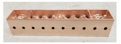
Figure 7. Complete brazed test block containing 10 cavities.
