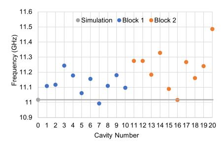
**Figure 10.** Frequency of all test cavities measured after printing. Simulated frequency is shown as horizontal grey line. Simulated geometry is adjusted to reflect cavity geometry before face machining.
