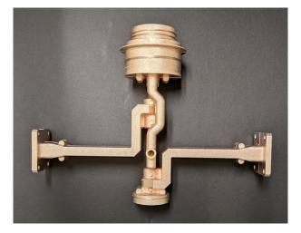
**Figure 1.** Complete klystron circuit with input and output waveguides, pump-out tubes, mounting for an electron gun and collector, and cavity tuning pins.
