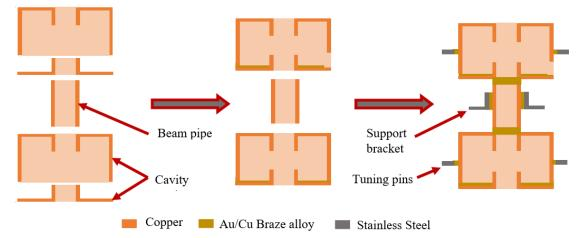
Figure 4. Diagram of conventional klystron circuit manufacturing process.
