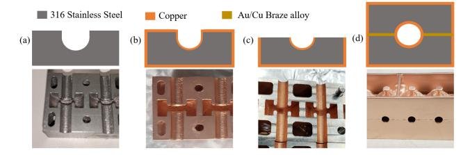
**Figure 5.** Diagram of proposed manufacturing process. (**a**) Printing, (**b**) Plating, (**c**) Face Machining, (**d**) Brazing.
