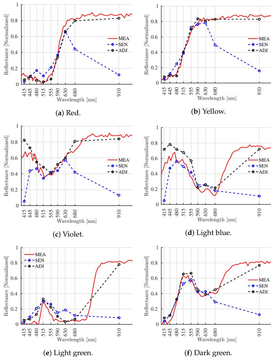
**Figure 9.** Validation with a reference method based on the use of a Yokogawa AQ6373 optical spectrum analyzer. MEA is the OSA reference reflectance. SEN is the raw reflectance, while ADJ is the best MLP setup-adjusted reflectance.
