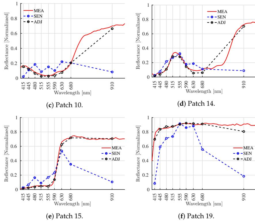
**Figure 8.** Comparison of the fits of multiple patches. MEA is the color checker reference reflectance. SEN is the raw reflectance, while ADJ is the best MLP setup-adjusted reflectance.
