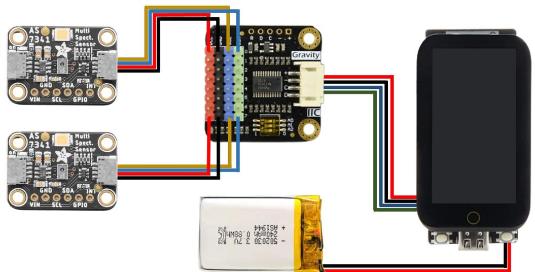
Figure 3. Electronic connection diagram.
