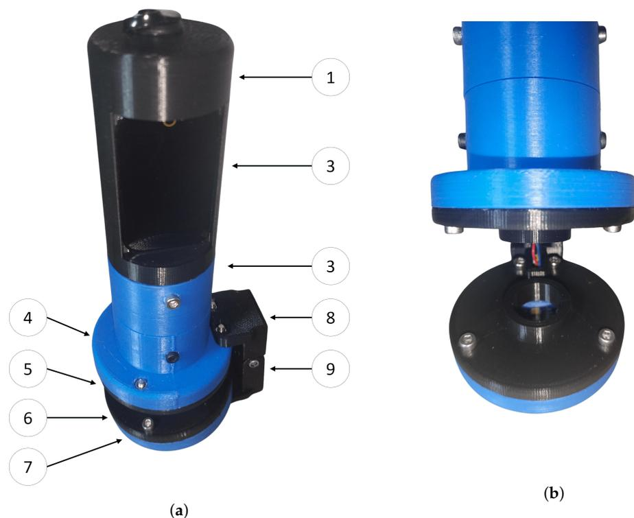
**Figure 7.** Photograph of the constructed spectrometer. (a) View of the entire device. (b) Detailed view of the area where the samples were located. The numbers in the figure correspond to the identification in the Figure 2.
