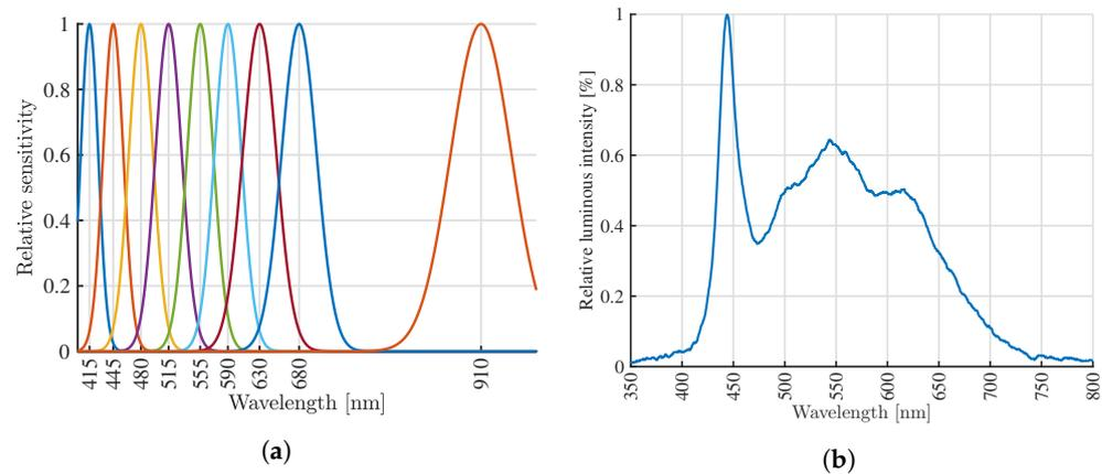
**Figure 1.** Relative sensitivity and luminous intensity in AS7341 integrated board. (a) Relative sensitivity of the AS7341. (b) Relative luminous intensity profile of the EAHC2835WD6 LED.
