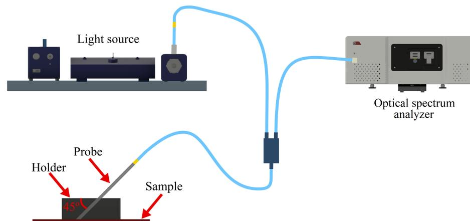
**Figure 6.** Experimental setup used to measure the reflectance with different colors using an OSA.
