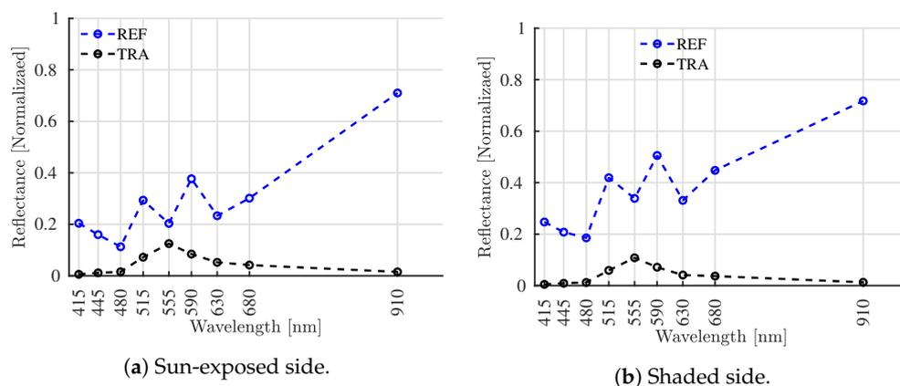
**Figure 10.** Measurements of transmittance and reflectance on a vegetable leaf.
