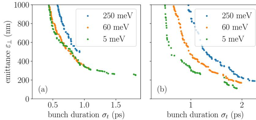
**Figure 2.** Pareto fronts of transverse normalized emittance and bunch duration for different MTEs using a Gaussian laser pulse (a) and a flat-top laser pulse (b). The optimization considers a 100 pC bunch charge.
