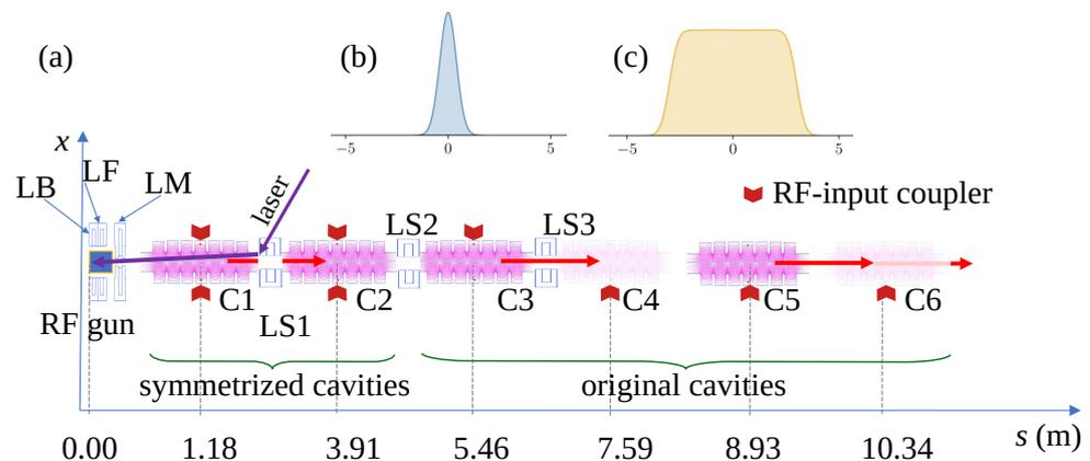
**Figure 1.** Diagram of the AWA photo-injector (a) and available Gaussian (b) and flat-top (c) temporal laser pulse distributions (the horizontal scale is in ps). In (a), the labels LB, LF, LM, and LS<sub>*i*</sub> represent solenoids, and C<sub>*i*</sub> represents the accelerating cavities. The red chevron symbols indicate the direction of the RF input couplers.
