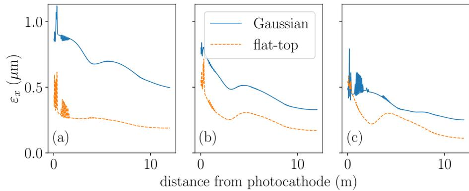
**Figure 3.** Emittance evolution along the AWA beamline for an MTE value of 250 (a), 60 (b), and 5 meV (c). The solid and dash traces correspond, respectively, to the case of a Gaussian and flat-top temporal shape for the photocathode laser pulse.
