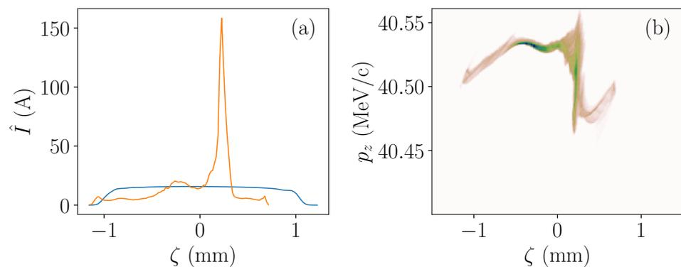
**Figure 7.** Initial (blue curve) and final (orange curve) peak current (a), along with the final longitudinal phase-space distribution (b), after magnetic bunch compression. The colormap used in the density plot (b) is the same as employed in Figure 4.
