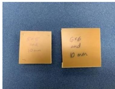
**Figure 8.** Sample detectors of different sizes. A detector size of 5 cm × 5 cm × 1 cm was used in the final version for both the laboratory tests and the Geant4 simulation.
