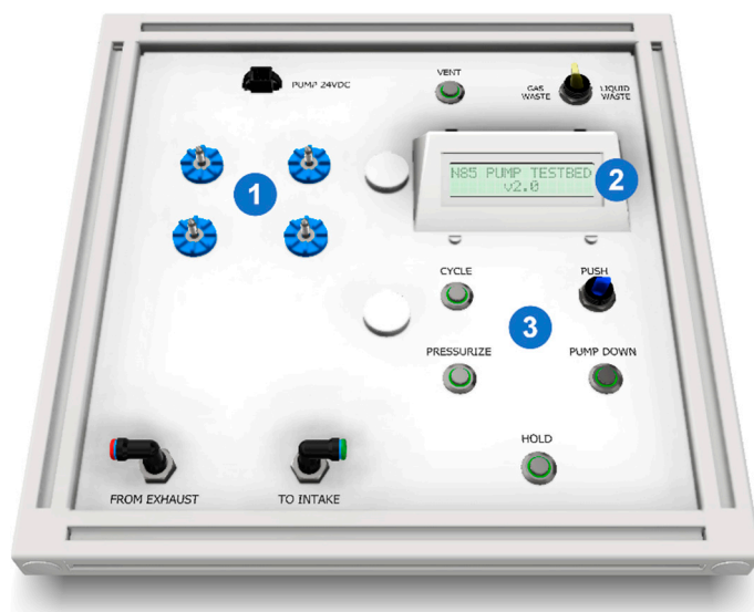
Figure 6. Lid subassembly featuring (1) captive panel screws and rubber vibration dampening grommets; (2) an LCD mounted on the bezel; and (3) illuminated controls.
