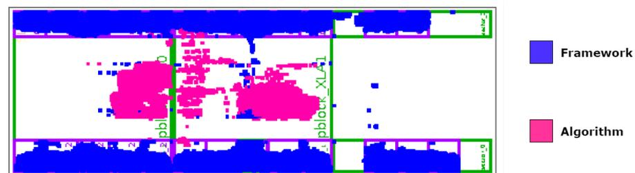
**Figure 5.** Calorimeter trigger algorithm floorplan for XCVU9P C2104 package FPGA. The trigger algorithms are placed in the middle of the SLR (magenta color). The firmware shell, which includes the MGTs firmware, is placed at the edges, which corresponds to the MGT ports (blue color).
