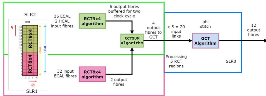
**Figure 7.** Integrated RCT and GCT algorithm block diagram. The RCT9x4, RCTSUM, RCT8x4, and the GCT phi stitch algorithms are implemented in SLR2, SLR1, and SLR0, respectively.
