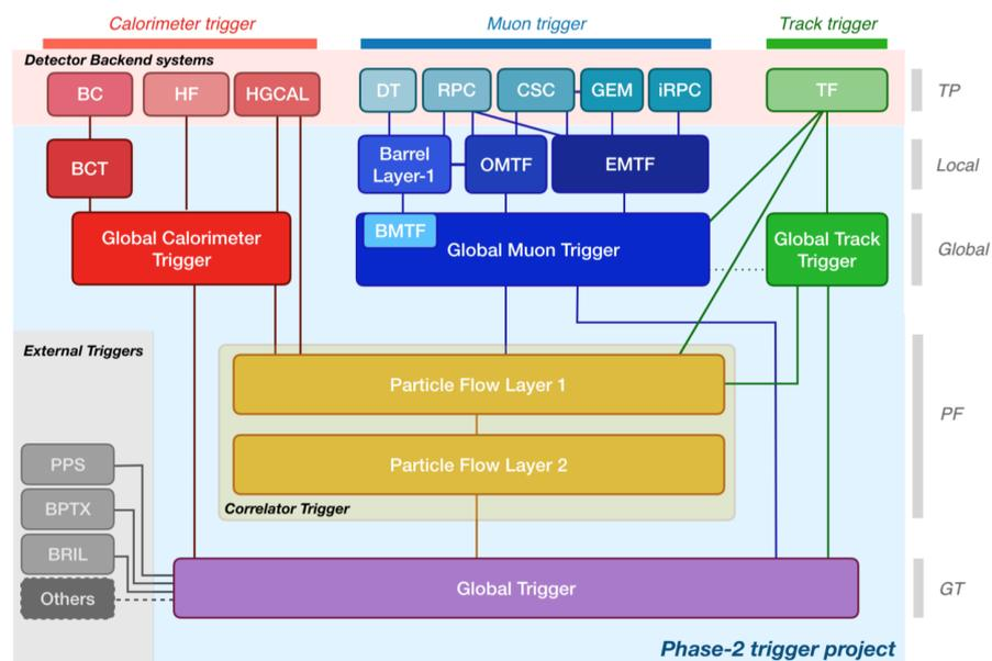
**Figure 2.** Block diagram of Phase-2 Level-1 trigger system [2]. It processes the information from sub-detectors, such as calorimeter, muon, and tracker. The trigger system is divided into five layers:
