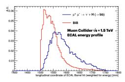
**Figure 1.** The (**left**) panel shows the time of the ECAL barrel hits with respect to bunch crossing time, for BIB and  $H \rightarrow \bar{b}b$  signal. In the (**right**) one the energy distribution of ECAL barrel hits as a function of the distance with respect to the beam axis is presented [1].
