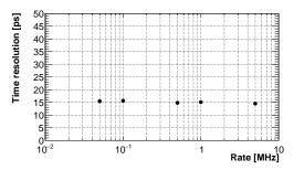
**Figure 9.** (**Left**): SiPM waveform in response to a laser pulse, sampled at 40 GS/s. Log-normal fit on the rising edge is overlaid. (**Right**): Effect of laser repetition rate on the time resolution.
