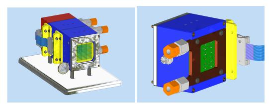
**Figure 7.** CAD 3D model of Crilin Prototype (Proto-1) on the (**left**). On the (**right**) a single module detail showing the cold plate heat exchanger mounted over the electronic board.
