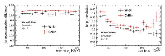
**Figure 3.** (**Left**): jet reconstruction efficiency as a function of the jet  $p_T$ , obtained by using the Crilin ECAL barrel and the W-Si ECAL barrel. (**Right**): jet  $p_T$  resolution as a function of the jet  $p_T$ , obtained by using the Crilin ECAL barrel and the W-Si ECAL barrel.
