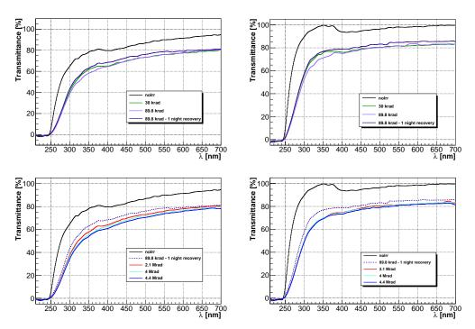
**Figure 5.** Transmission spectra obtained in the different irradiation steps for the naked crystal (**top** and **bottom left**) and the crystal with Mylar wrapping (**top** and **bottom right**).
