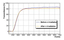
**Figure 6.** Transmission spectra obtained after the irradiation at FNG with 14 MeV neutrons for a total fluence of  $10^{13}$ n/cm<sup>2</sup> (orange line) compared with the results after the 16 hours optical bleaching (blue line) for the naked crystal (**left**) and for the crystal with Mylar wrapping (**right**).
