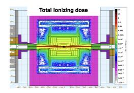
**Figure 4.** (**Left**): Map of the 1-MeV-neq fluence in the detector region for a Muon Collider operating at  $\sqrt{s} = 1.5$  TeV with the parameters described in [3], shown as a function of the position along the beam axis and the radius. (**Right**): Map of the TID in the detector region shown as a function of the position along the beam axis and the radius.
