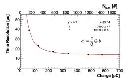
Figure 10. Effect of sampling frequency on time resolution (left). Time resolution as a function of charge and  $N_{p.e.}$  (right).
