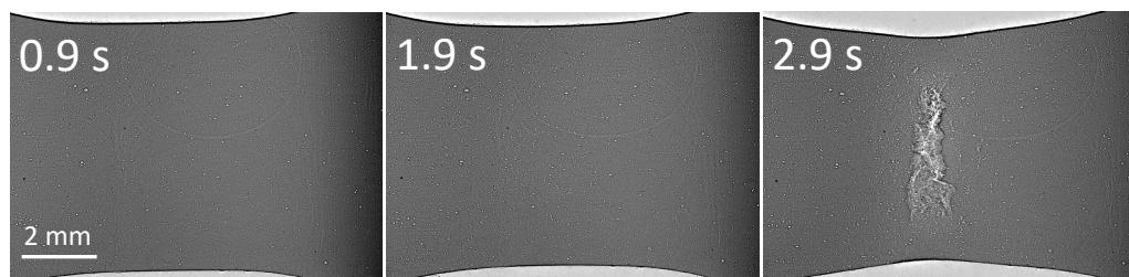
**Figure 5.** X-ray images of Scalmalloy specimen (printed 0° flat) under tension in quasi-static UTM. Image series captured by Photron SA-Z high speed camera at 10 kHz frame rate and a resolution of  $1024 \times 1024$  pixels. From left to right, different timestamps capturing the formation of voids to fracture. White contrast in these radiographs represent high intensity X-rays. The aspect ratio of the images are adjusted for illustration purposes.
