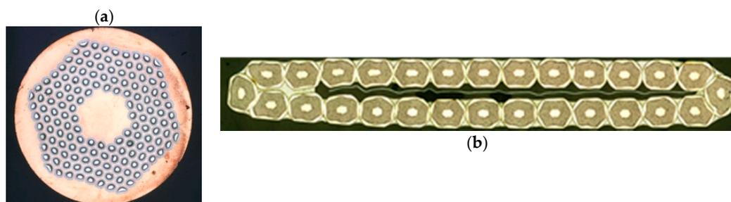
**Figure 1.** (a) Cross section before heat treatment of 150/169  $Nb_3Sn$  wire of the Restacked Rod Process<sup>®</sup> type [10]. (b) Cross section of 28-strand Rutherford cable [12].
