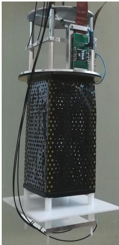
**Figure 3.** The Bern field-shell demonstrator LArTPC. The field-shell and cathode are made from  $\sim 50 \mu\text{m}$  resistive kapton foil. For this test, the field-shell was perforated to allow the purification of the LAr within the active volume. The Time Projection Chamber (TPC) has a  $7 \text{ cm} \times 7 \text{ cm}$  footprint and a 15 cm drift length. A bias of up to  $-23 \text{ kV}$  was applied to the cathode to generate a  $1.5 \text{ kV cm}^{-1}$  drift field [34].
