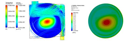
Figure 4. (a) Example of simulated flow streamlines and temperatures; and (b) stresses in the target entrance window for a 100  $\mu$ A, 20 mm beam.
