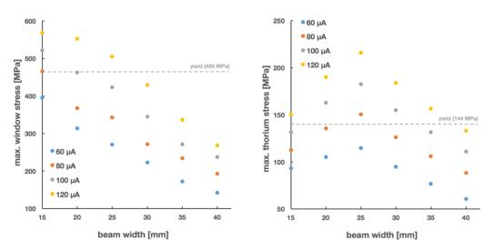
**Figure 6.** Maximum simulated stresses resulting from temperatures within window (**left**) and thorium (**right**) target components during irradiations. Please note that increase in thorium foil stresses as beam width increases (from 15 to 25 mm) is due to deposition of heat in regions of the thorium that are not in contact with the window.
