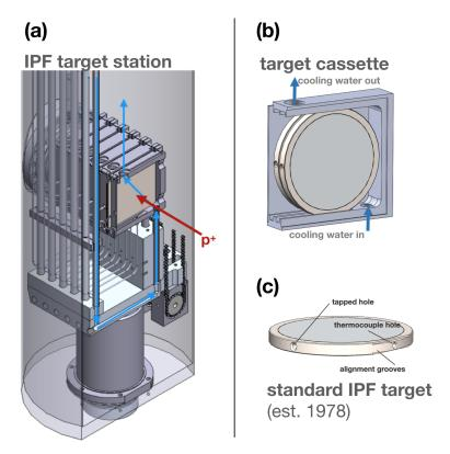
**Figure 1.** (a) IPF target station at beam level, with six cassettes inserted into the beam. The arrows indicate cooling water flow direction; (b) An IPF cassette holding two targets; (c) A typical IPF target.
