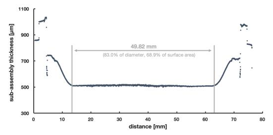
**Figure 3.** Plot of the thorium target sub-assembly thickness. Measurement of the inward deflection of the window, as also seen in Figure 2*c*, indicates the region for which the thorium and windows are in contact. The expected thickness in the centre of the sub-assembly (assuming contact of the thorium with both windows) is  $504 \mu m$ .
