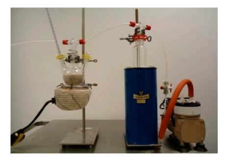
Figure 4. Condensation unit for the recovery of [<sup>18</sup>O]-water from azeotropic mixtures.
