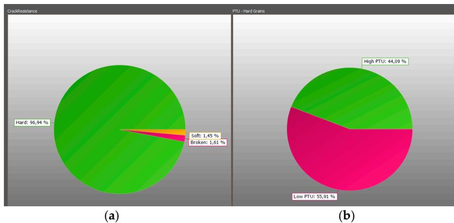
Figure 9. (a) Crack resistance parameters of Hard (green), broken (BBF) (pink) and Soft (orange) kernels; and (b) PTU in hard kernels, which can be High PTU (green) or Low PTU (pink).
