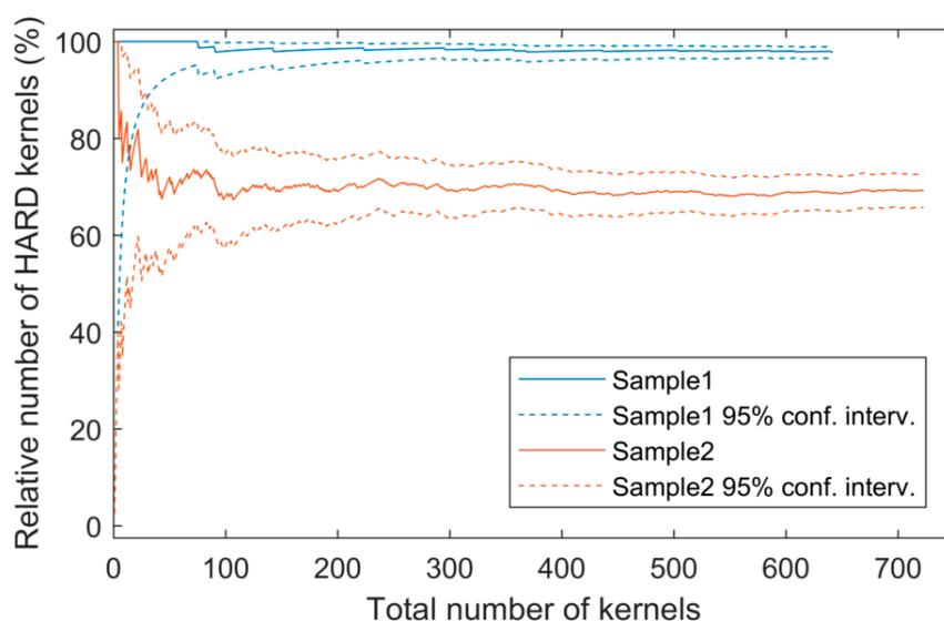
**Figure 5.** Percentage of Hard kernels vs. the total numbers of kernels for two samples with two different qualities. The 95% confidence intervals are marked with dotted lines. Note that the confidence intervals decrease with the number of kernels.
