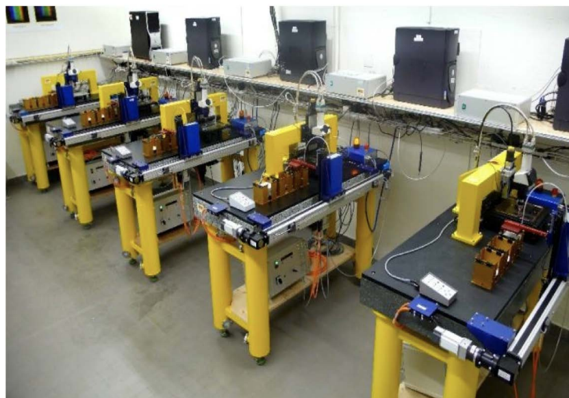
Figure 8. The six automated scanning microscopes of the University of Bern equipped with automated film exchangers. They feature a total scanning speed up to 180 \text{ cm}^2 emulsion surface per hour.
