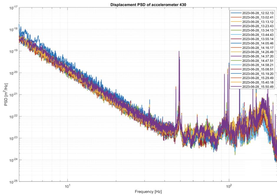
**Figure 7.** The results of a long-term measurement of the environmental noise in the laboratory is shown. The plot reports multiple measurements performed with one accelerometer and taken at consecutive times.
