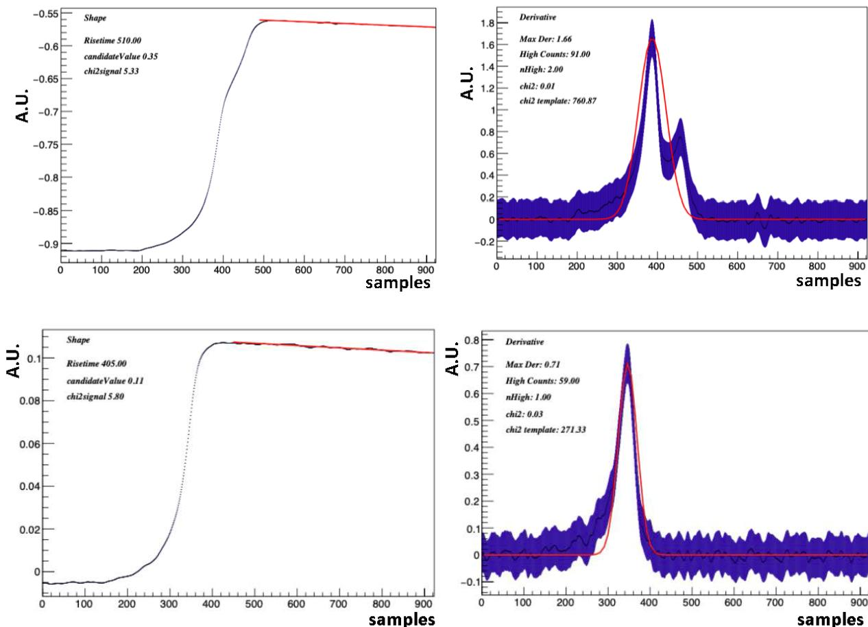
**Figure 1.** Top panel: a typical multi-site event that would survive selection cut 2 but not selection cut 3. Bottom panel: a signal event that has been selected by the algorithm. Figures on the right correspond to the derivatives of the corresponding curves on the left. The full acquisition time window is 2560 ns, one acquisition corresponds to 1024 samples, and the sampling rate is 400 MHz, so one sample corresponds to 2.5 ns.
