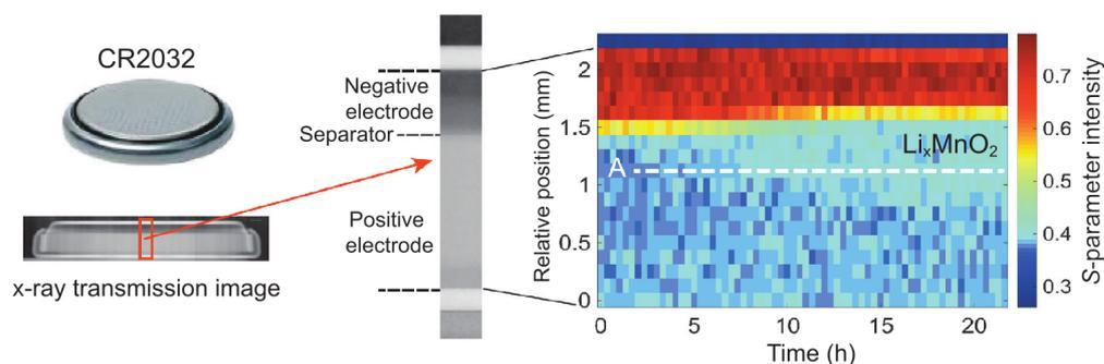
**Figure 3.** Compton scattering intensity as a function of time during the discharge of the CR2032 commercial battery. Red and blue regions correspond to the negative electrode and the  $\text{Li}_x\text{MnO}_2$  in the positive electrode, respectively. The olefin separator is marked with yellow. The battery was discharged under a constant current of 5.5 mA for 15.75 h. Adapted from Ref. [37].
