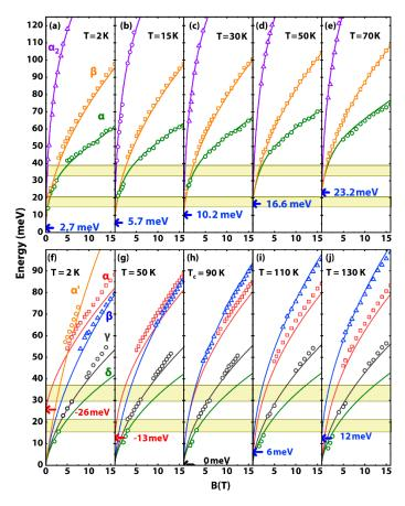
**Figure 2.** Fan chart of inter-LL transitions in 6-nm wide  $HgTe/Cd_{0.62}Hg_{0.38}Te QW$  (**a**–**e**) and 8-nm wide width  $HgTe/Cd_{0.8}Hg_{0.2}Te QW$  (**f**–**j**) from work [11]. The calculated transitions are shown in solid lines while the experimental data are represented by the open symbols in the same colors as the theoretical curves. The estimated values of the energy gap are shown by the horizontal arrows. Shaded areas indicate the GaAs and HgCdTe reststrahlen bands.
