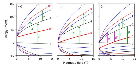
**Figure 1.** Landau levels of HgTe/Cd<sub>0.7</sub>Hg<sub>0.3</sub>Te QW calculated within axial approximation for: (**a**) band insulator (d = 5.5 nm); (**b**) zero-gap semiconductor (d = 6.3 nm); (**c**) topological insulator (d = 7.4 nm). Zero-mode LLs are shown with bold lines. LL indices are shown with both numbers on the lines and line colors. We use the same calculation method and LL indices notation of as in [8,9].
