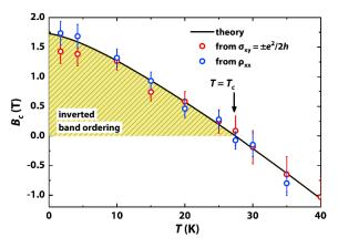
**Figure 5.** Theoretical (black curve) and experimental (open symbols) values for critical magnetic field as a function of temperature for 6.5 nm HgTe/Cd<sub>0.65</sub>Hg<sub>0.35</sub>Te QW from work [13].
