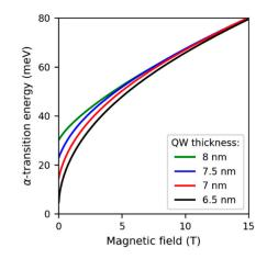
Figure 3. Calculated energy of  $\alpha$ -transition for HgTe/Cd<sub>0.7</sub>Hg<sub>0.3</sub>Te QWs of different thickness.
