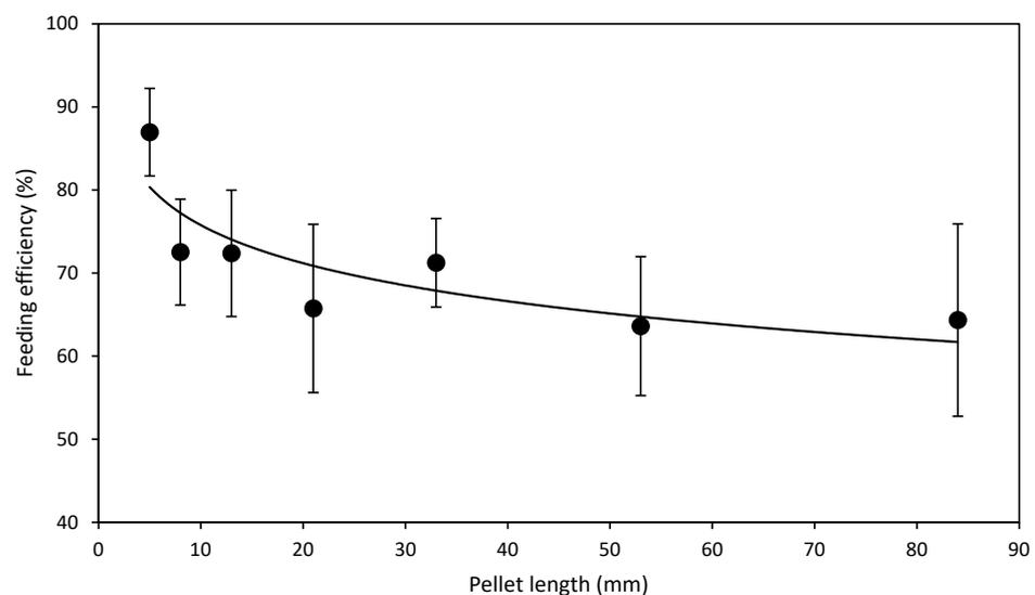
**Figure 5.** Effect of pellet length on hard and dry pellet (HDP) feeding efficiency, the line shows logarithmic regression  $y = -6.6\ln(x) + 91.0$ ,  $R^2 = 0.075$ ,  $p = 0.041$ . Values are average, error bars denote S.E.
