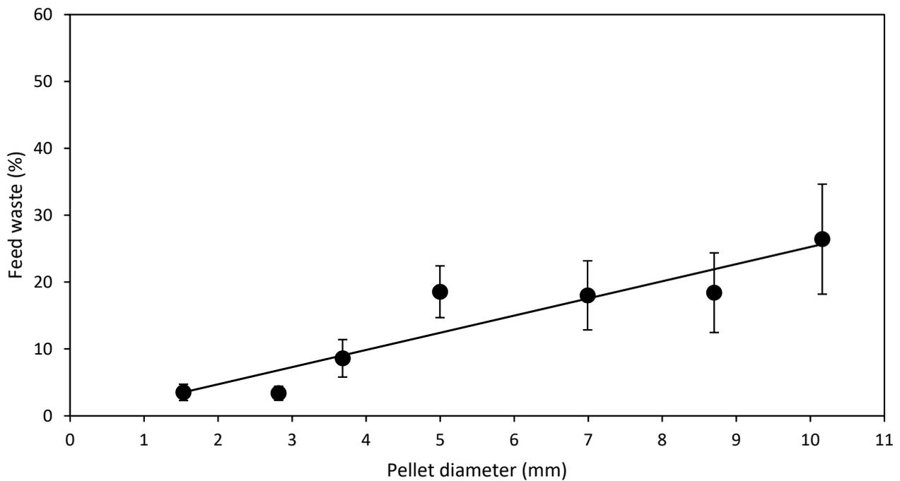
**Figure 2.** Effect of pellet diameter on soft and moist pellet (SMP) feeding related waste (FRW). The line shows linear regression for FRW  $y = 0.26x - 0.4$ ,  $R^2 = 0.26$ ,  $p = 0.000$ . Values are average, error bars denote S.E.
