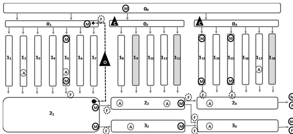
**Figure 7.** Fish farm general layout (A: paddle-wheel aerator, C: oxygen cone; O: high pressure oxygenator; M: physico-chemical monitoring location; F: water flow monitoring location). Some ponds (i.e., 1<sub>9</sub>, 1<sub>12</sub> and 1<sub>18</sub>) were not stocked at the moment of monitoring, they are represented in grey. The figures 0, 1, 2 and 3 are theoretical numbers of water uses.
