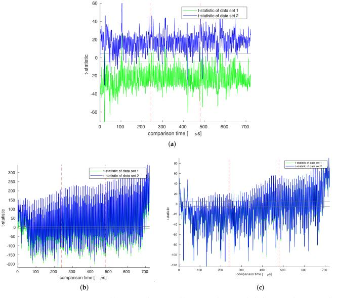
**Figure 6.** (a) TVLA results on AES. (b) TVLA results on AES locked using 128-bit Anti-SAT locking key (#CKB = 64). (c) TVLA results on AES locked using 128-bit SFLL locking key (#CKB = 29).
