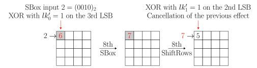
**Figure 7.** Propagation of wrong logic-locking key bits over two AES operations. The introduced errors are shown in red to demonstrate the effect of a wrong logic-locking key bit canceling out the effect of another.
