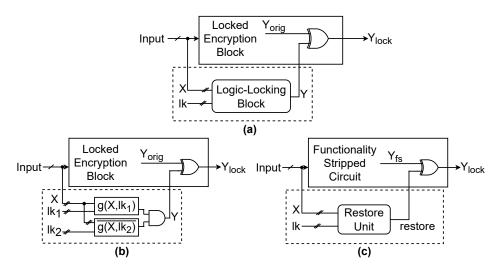
Figure 3. (a) Generic point function-based logic locking (b) Anti-SAT (c) SFLL.
