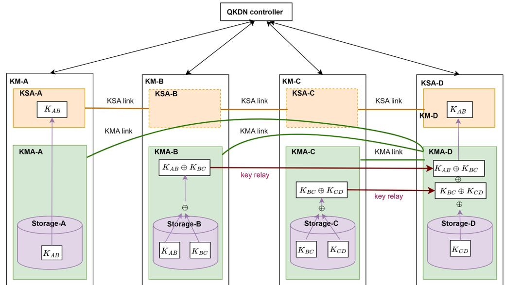
Figure 5. Quantum-key bit forwarding through a direct link between the first repeater node and the destination node.
