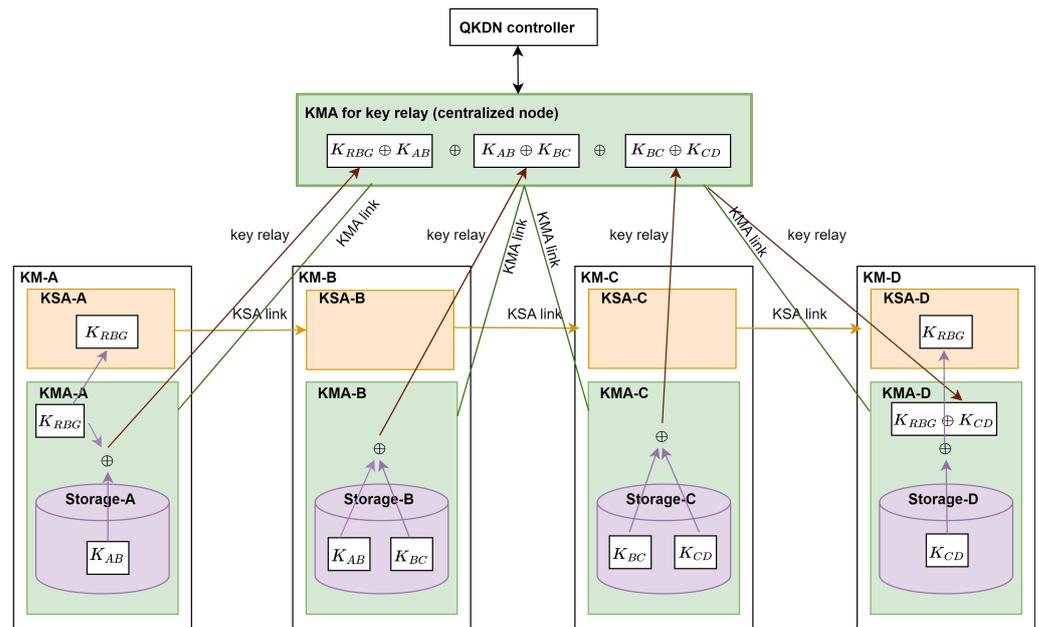
Figure 6. An optimal approach for forwarding quantum key bits by using a centralized controller.
