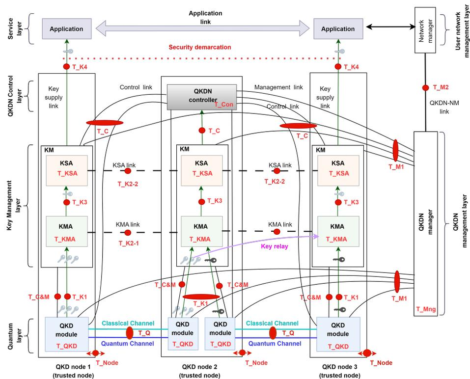
**Figure 1.** The functional diagram of a QKDN performing key relay, in which the elements belonging to the attack surface and their threats are highlighted in red (adapted from [41,42]). Dotted black lines represent KSA and KMA links. Blue and light blue lines depict, respectively, quantum and classical channel. Quantum key bits provided to applications are shown in grey, whereas black keys denote quantum key bits used for key relay.
