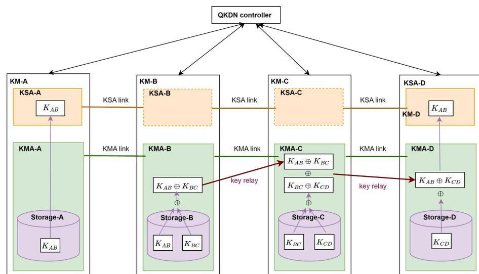
Figure 4. A naive approach to quantum key bit forwarding.
