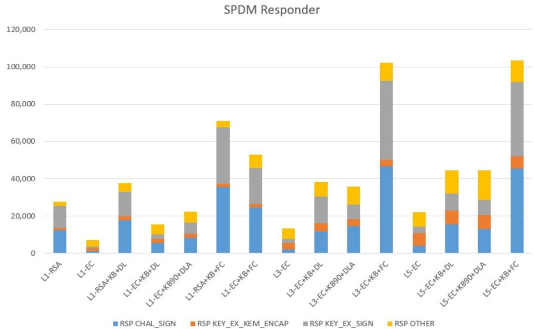
Figure 7. SPDM responder performance—Kyber, DILITHIUM, FALCON (microsecond).
