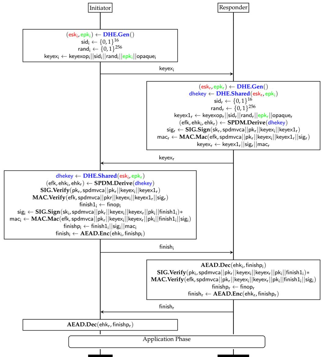
Figure 2. Traditional SPDM DHE-based key exchange flow.
