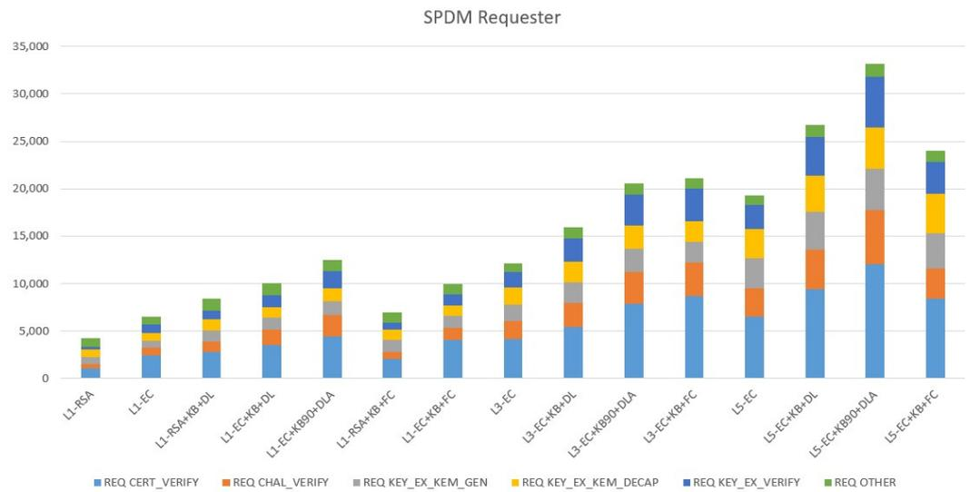
Figure 5. SPDM requester performance—Kyber, DILITHIUM, FALCON (microsecond).
