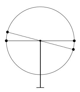
Figure 5. Circular motion of an equal-arm balance.
