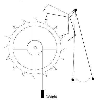
Figure 1. Simplified diagram of an escapement mechanism.
