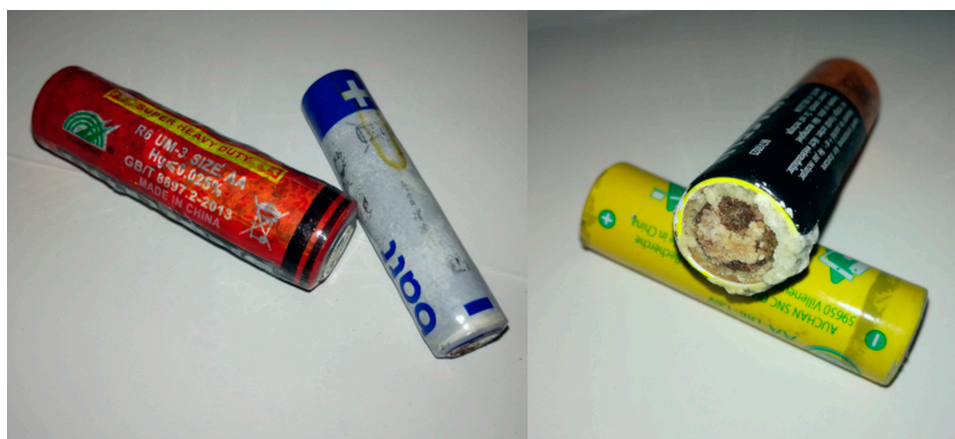
Figure 13. Some alkaline batteries immediately discharged because visibly damaged; four different brands.
