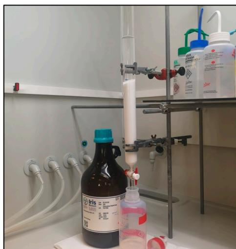
**Figure 1.** DCM drying process with the use of a basic aluminum oxide column.
