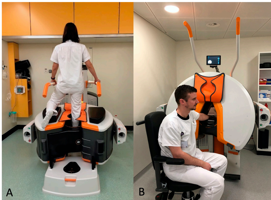
Figure 2. Upright position in the WB CBCT to investigate the foot, ankle, or knee, (A) and sitting position with arm extended to explore the hand and wrist (B). WB: weight-bearing; CBCT: cone-beam computed tomography.
