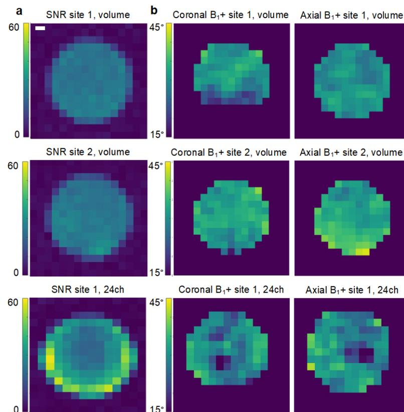
**Figure 1.** Comparison of the coils used at the two sites. The tests were performed on a natural abundance dimethyl silicone phantom by excitation of a single resonance with an echo-planar imaging readout. The signal-to-noise ratio (SNR, (a)) was determined over a 5 min scan. The  $B_1^+$  profile (b) was determined using the double angle method. The white scale is 2 cm.
