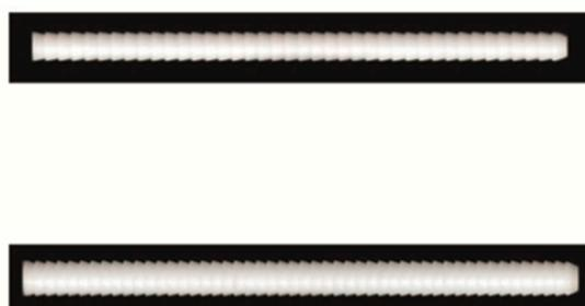
**Figure 1.** Two bioabsorbable pins with diameters of 2 mm (**top**) and 3 mm (**bottom**) were used. The pins, forged with 30% HA and 70% PLLA, are bioactive and bioabsorbable.
